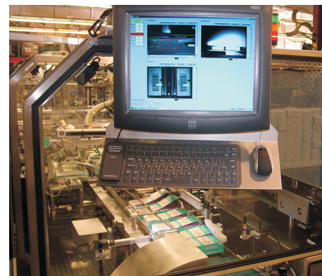
Vision system and machine discharge modul (below)
